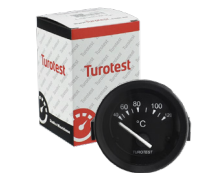
TU300476 ELÉTRICO PRETO 52MM 12V 40°C (69 OHMS) A 120°C (7 OHMS) MWM
