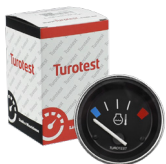
TU302385 ELÉTRICO 60MM 12V 40°C (360 OHMS) A 110°C (70 OHMS) MF200 MF275 MF292 MF265 MF295 MF296 MF297 MF299
