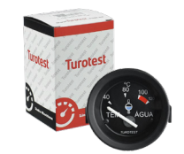
TU300473 ELÉTRICO PRETO 52MM 12V 40°C (325 OHMS) A 120°C (60 OHMS) MF1630 MF3366 MF3640
